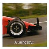
Each car carries a small vertical blade at the front called a timing strut. As a car approaches the start, the marshals line the car up immediately behind the timing beam. A chock behind the rear wheel keeps the car in the right position. When the driver is given the green light, they start in their own time. As the car moves forward it breaks the light beam and starts the electronic timing equipment.
